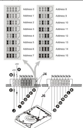
The drive has two option jumper blocks designated as 'J-4' and 'J-6' located on the circuit board.
